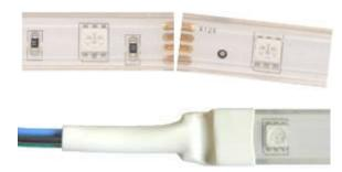
Be careful when soldering that you do not overheat the pads as this heat can damage the pad and the LEDs, a small dab of flux paste helps with a fast solder connection. **Make sure the wire you use is rated for load.**
