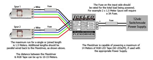
Next you will need to connect the 12vdc power supply to the Flexidriver.
